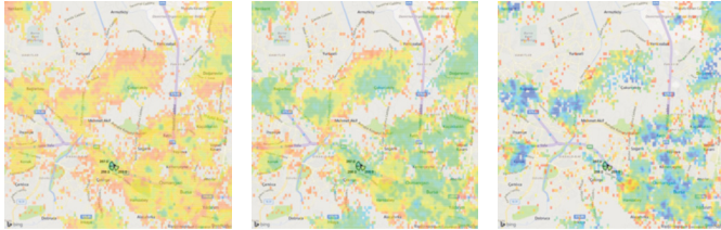
Geo-located customer experience (signal strength/quality and too many server) maps, created for single site verification
