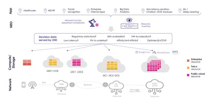
Figure 2: 5G Network Function Placement
