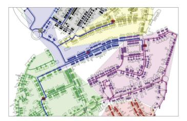
GIS based fiber planning tools can improve design accuracy. This is a plan view of the street topology with color coded distribution areas (image courtesy of FiberPlanIT)
