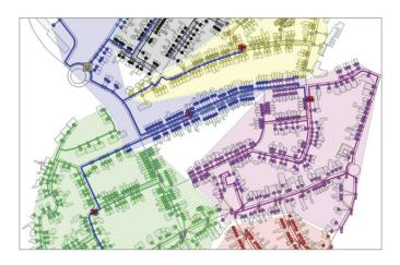
GIS based fiber planning tools can improve design accuracy. This is a plan view of the street topology with color coded distribution areas (image courtesy of FiberPlanIT)
